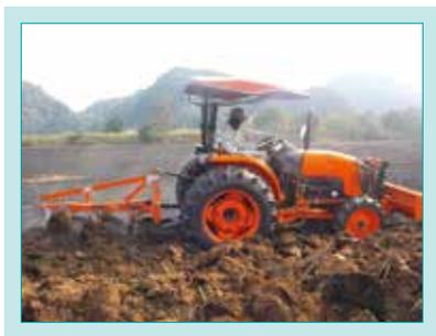
Fig. 6 Disk Plow Operation
