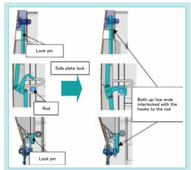
Fig. 8 Locking Mechanism
