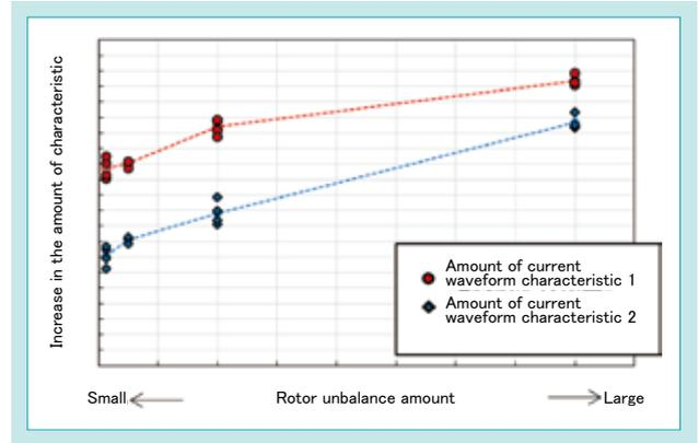
Fig. 8 Effect of Pump Rotor Unbalance
