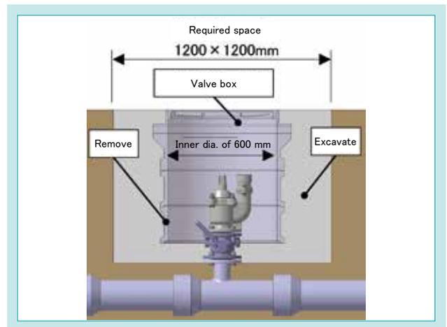
Fig. 4 Space Required for Conventional Method
