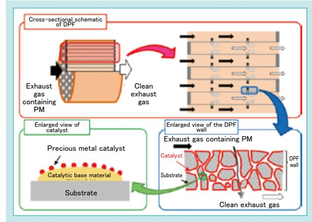
Fig. 2 Schematic Diagrams of a DPF
