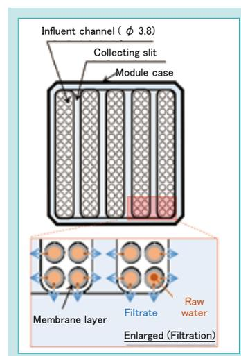
Fig. 2 Cross-section of the Flow Path
