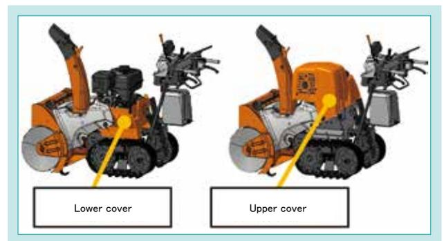
Fig. 3 Engine Cover Structure
