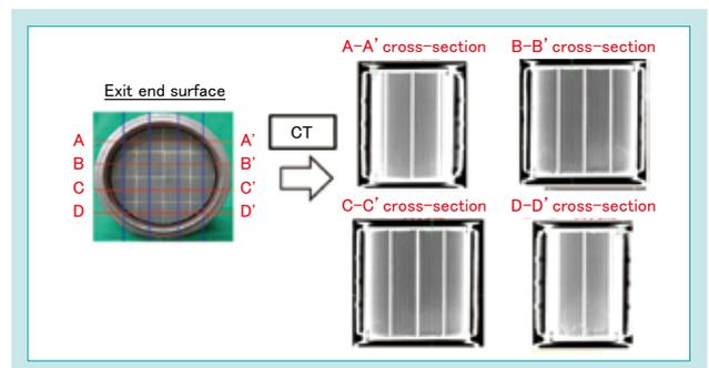
Fig. 7 CT Images for the DPF After Diesel Engine Endurance Test
