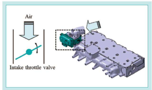
Fig. 7 Intake Throttle Valve
