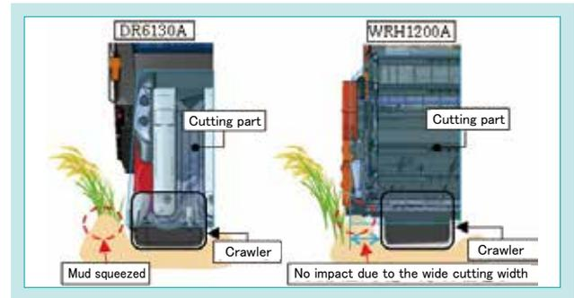
Fig. 10 Relative Position Between Reaper and Crawler
