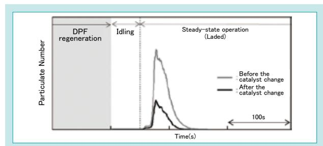
Fig. 11 PN after DPF Regeneration Before and After Improving the DPF Catalyst
