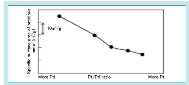
Fig. 15 Surface Area for Noble Metal and Pt/Pd Ratio
