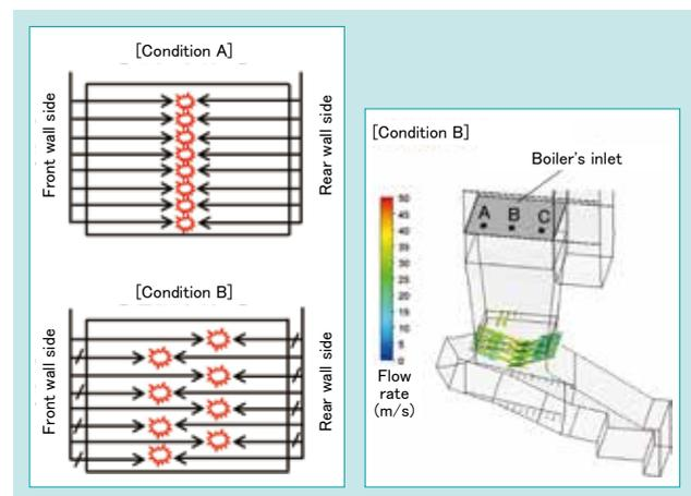
Fig. 9 Comparison of Two Secondary Air-injection Methods
