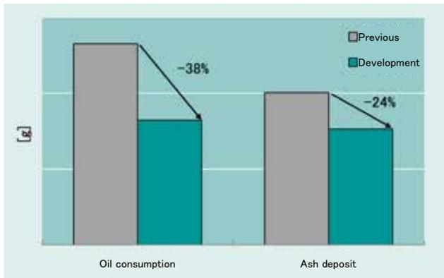
Fig. 9 Reduction of Oil Consumption and Ash Deposits
