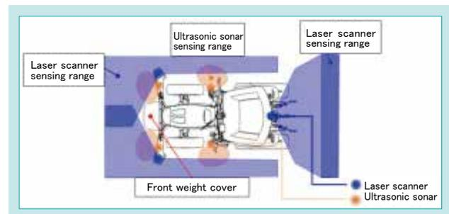
Fig. 9 Object Detection System
