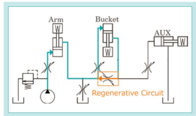
Fig. 16 Hydraulic Circuit 5(AMV)
