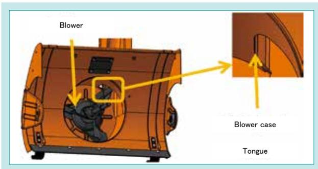
Fig. 5 Snow Removal Part Analysis Model
