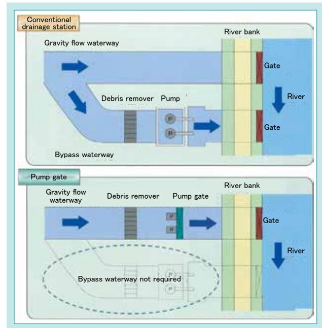
Fig. 2 Shape of Conventional Drainage Pump Station and Pump Gate
