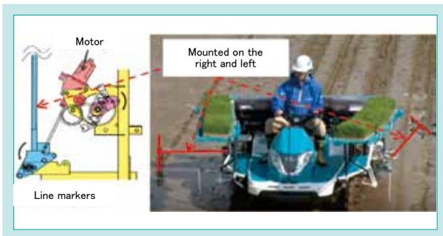
Fig. 5 Line Marker for Medium and Large Class
