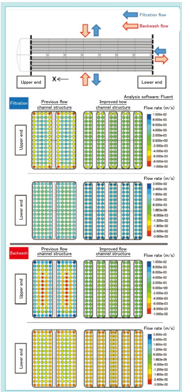
Fig. 4 Velocity Contour of Each Channel Section
