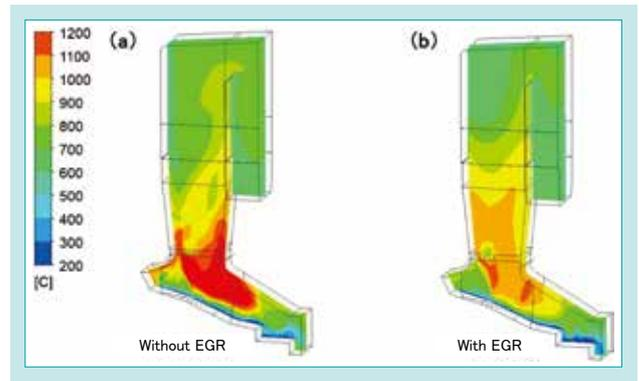
Fig. 5 Comparison of Temperature Distribution in Incinerator
