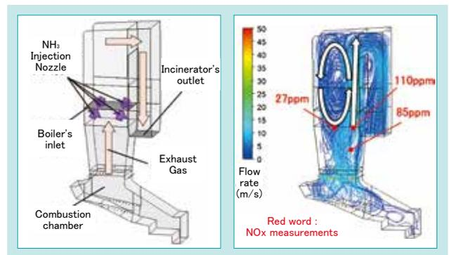
Fig. 6 Scheme of SNCR Test in Actual Incinerator
