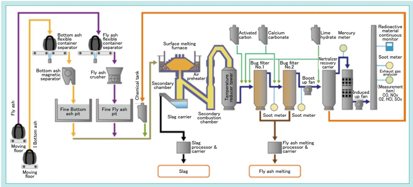
Fig. 3 Processing Flow of Temporary Ash Treatment Facility
