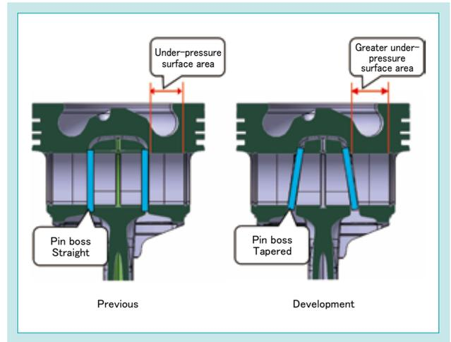
Fig. 6 Tapered Pin Boss
