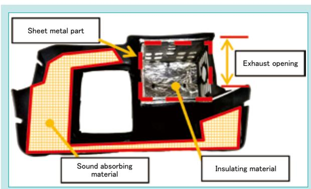
Fig. 4 Engine Top Cover Internal Structure
