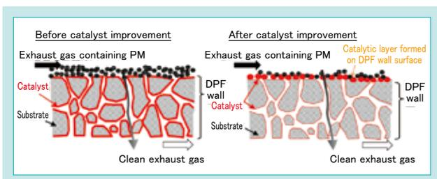
Fig. 9 Schematic Diagrams Before and After Improving the DPF Catalyst
