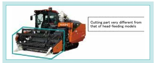
Fig. 3 Autonomous Driving Assist Combine Harvester WRH1200A
