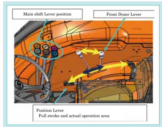
Fig. 10 Positioning of Operating Levers
