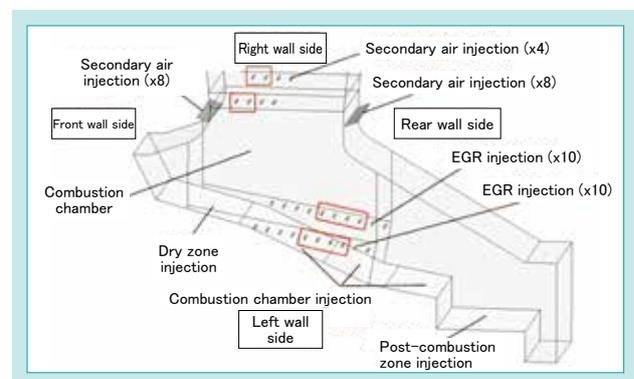
Fig. 4 Positions of Gas Injection Ports
