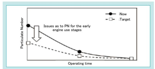
Fig. 13 Operating Time for a Diesel Engine and PN over RMC
