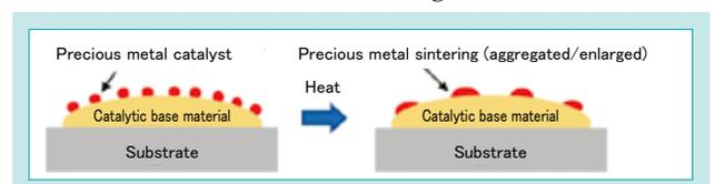
Fig. 14 Schematic Diagrams on Thermal Deterioration for DPF Catalyst
