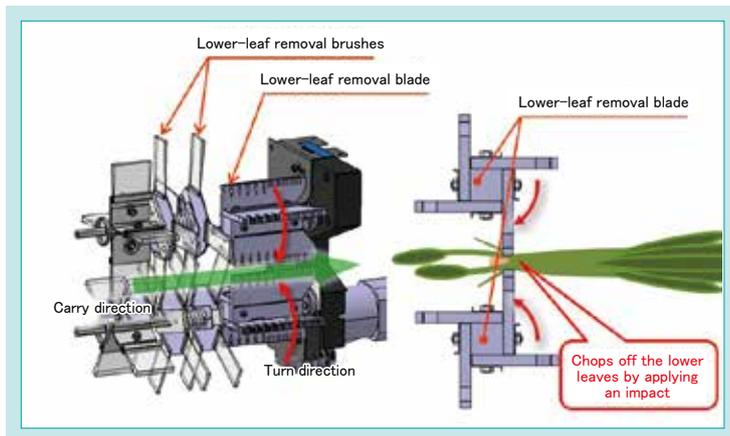
Fig. 9 Mechanism of “NC301” for Removing Cotyledons and Lower Leaves
