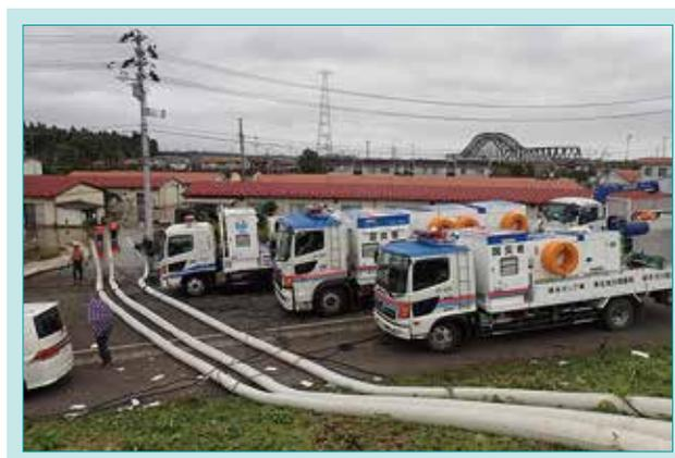
Fig. 1 Drainage Pump Vehicles Operating Photo
