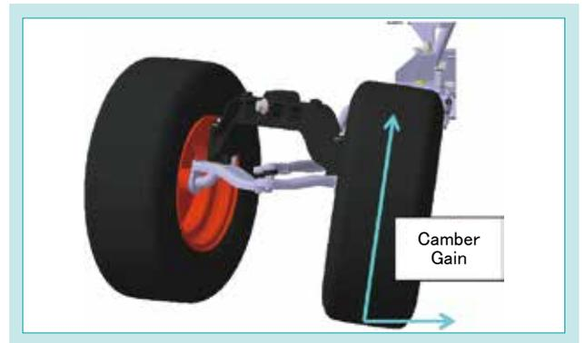
Fig. 10 T90 Camber Gain in a Turn
