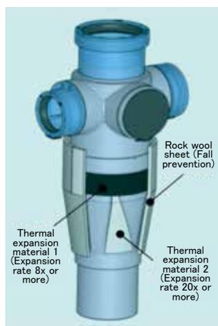
Fig. 1 Composition of Refractory Material
