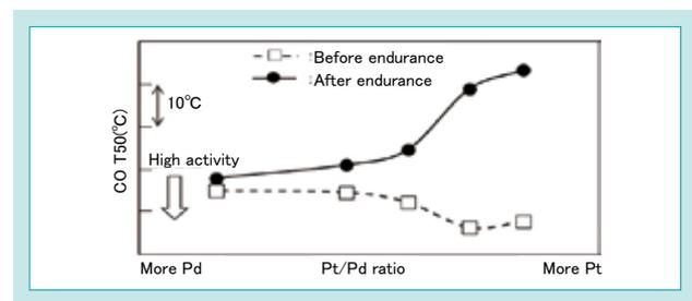
Fig. 16 CO Oxidation Activity and Pt/Pd Ratio
