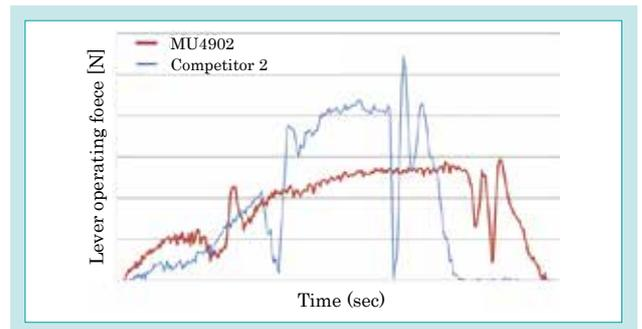
Fig. 9 Operating Force of Shuttle Lever
