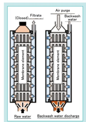
Fig. 3 Internal Flow of the Module
