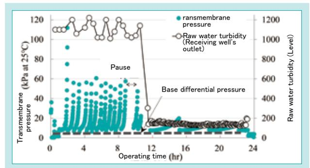
Fig. 7 Transmembrane Pressure During High Turbidity Test
