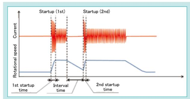
Fig. 6 Current and Rotational Speed at Pump Start-up
