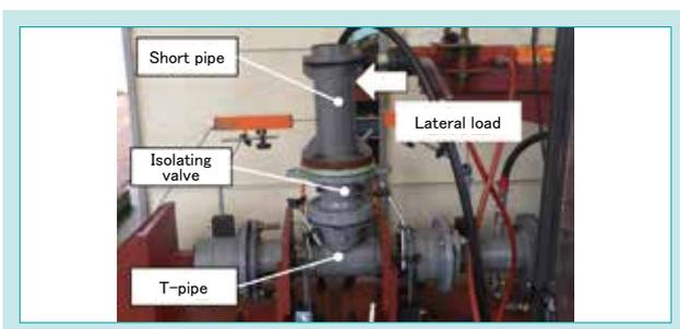
Fig. 8 Aspect of Lateral Load Test
