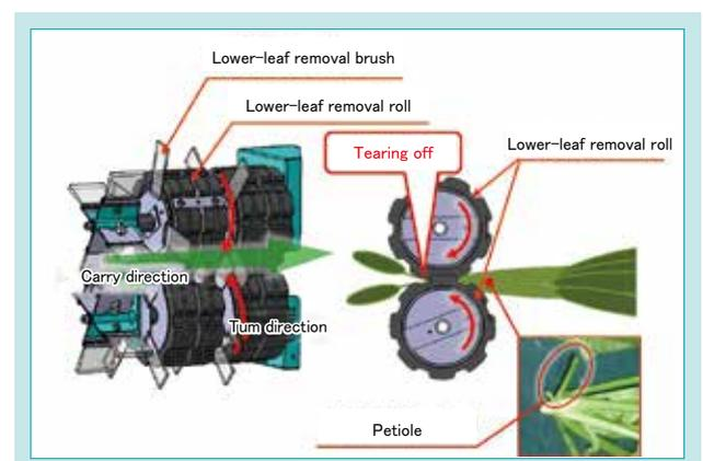
Fig. 6 Mechanism of “NC300” for Removing Cotyledons and Lower Leaves
