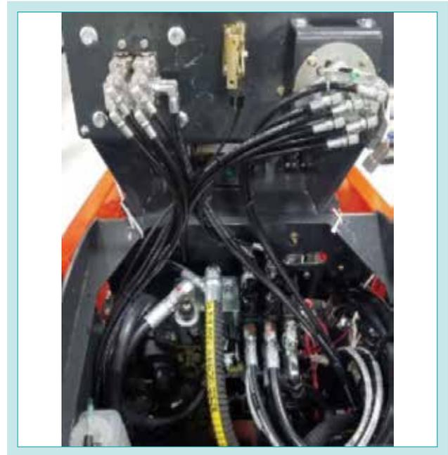
Fig. 3 Hydraulic Hose Routings
