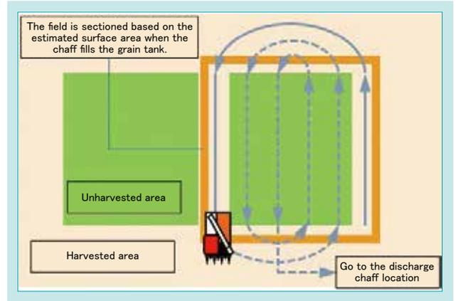
Fig. 13 Automatic Setting Area Using Yield Prediction
