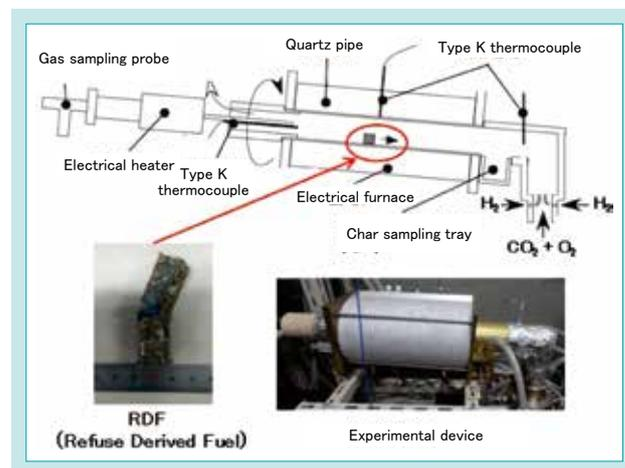
Fig. 2 RDF Combustion Test Device
