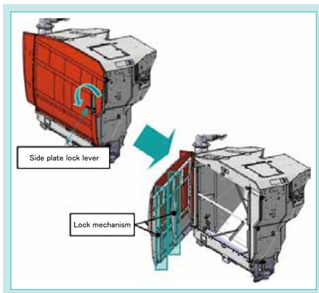
Fig. 7 Easy Maintenance of Grain Tank
