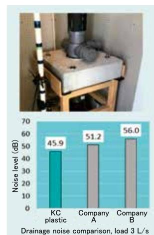
Fig. 4 Noise Measurement Result
