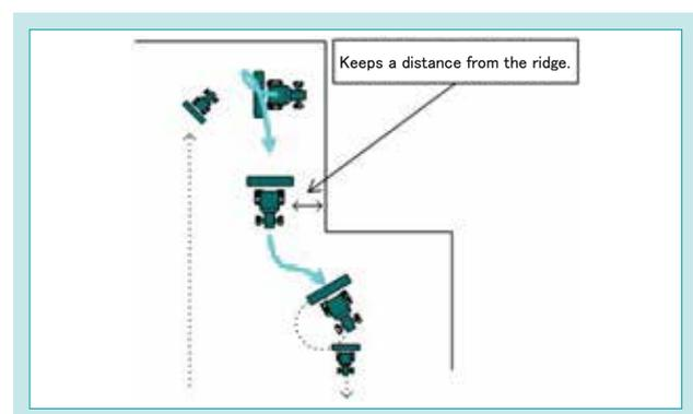
Fig. 4 Turning Route Along the Ridge
