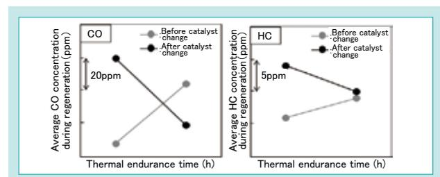
Fig. 19 CO and HC Emissions During DPF Regeneration
