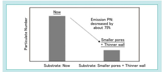
Fig. 5 PN over RMC Before and After Improving DPF Substrate
