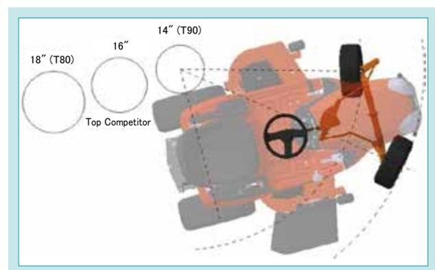
Fig. 7 Turning Radius Comparison
