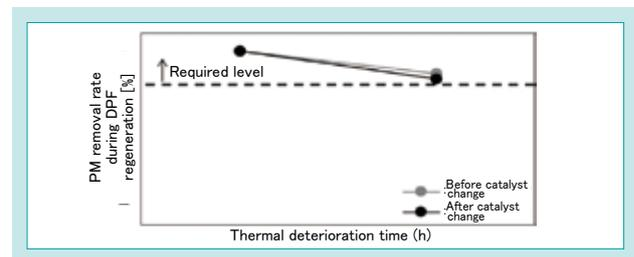
Fig. 18 PM Removal Ratio by DPF Regeneration
