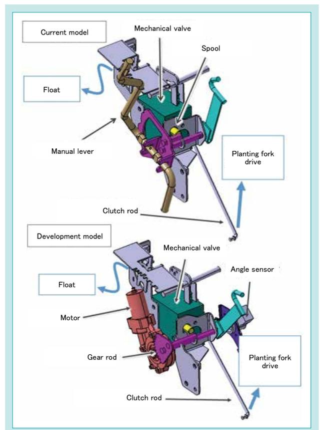
Fig. 4 Electrification Mechanism of Planting Part
