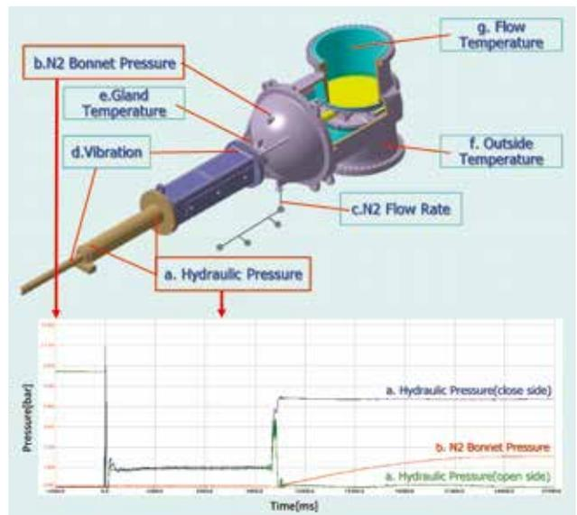
Fig. 4 Extracted Target Data for Measurement
