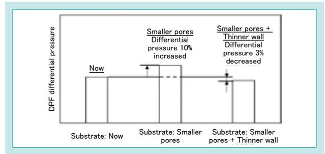
Fig. 4 DPF Differential Pressures Before and After Improving the DPF Substrate
