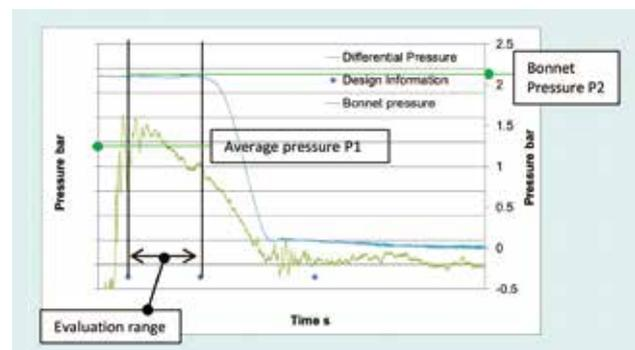
Fig. 6 Evaluation Factor for Valve Sealing Function
