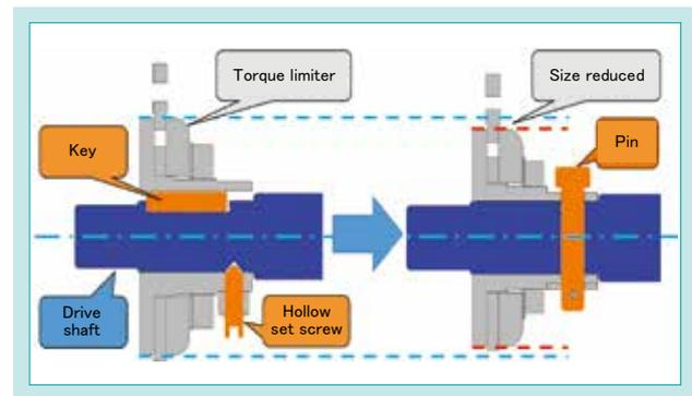
Fig. 10 Considering Miniaturization of Torque Limiter
