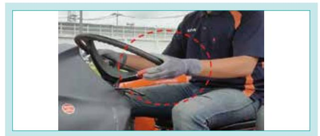
Fig. 8 Position of Shuttle Lever
