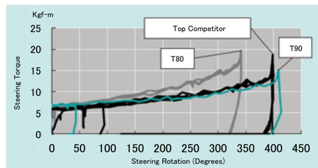
Fig. 13 T90 Steering Force Comparison
