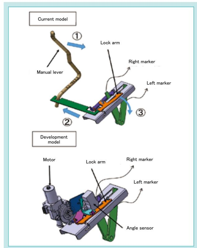
Fig. 6 Electrification Mechanism of Line Marker
