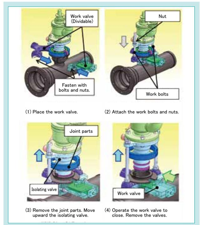
Fig. 10 Replacement Method Procedure
