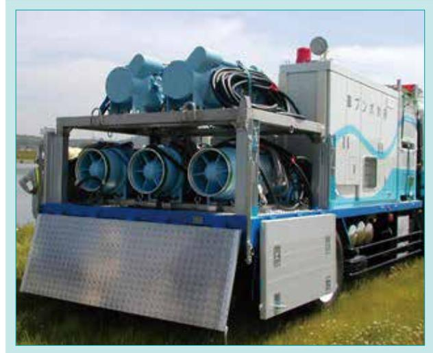
Fig. 2 Early Drainage Pump Vehicle
