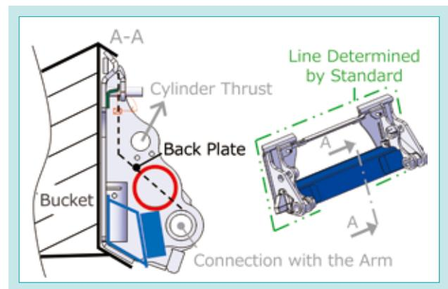
Fig. 10 Structure of Hitch
