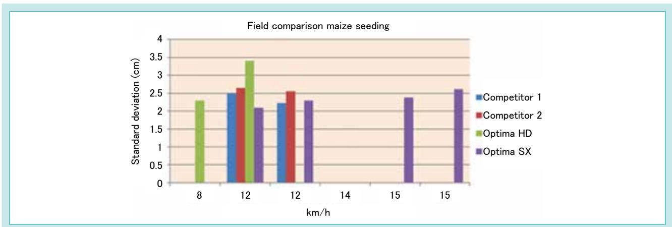
Fig. 23 Standard Deviation of Placing
