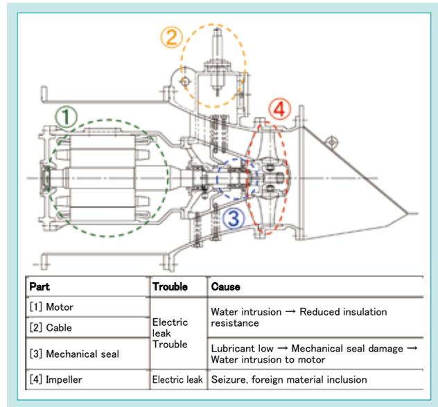
Fig. 5 Major Pump Failure Parts and Causes
