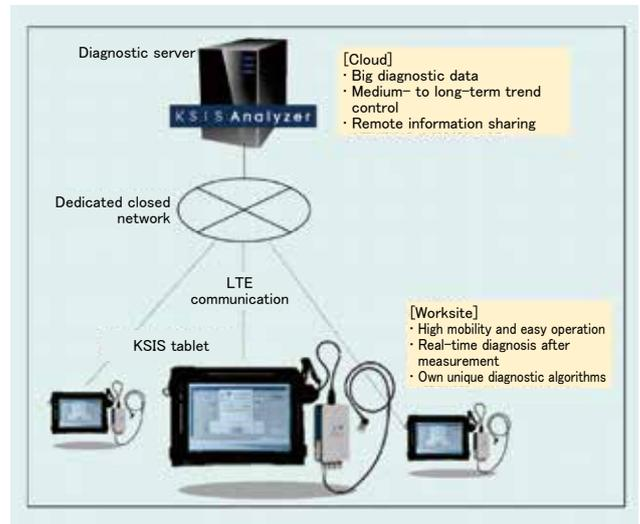
Fig. 9 KSIS Platform System Diagram
