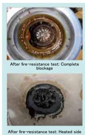
Fig. 2 Situation After Fire Resistance Test
