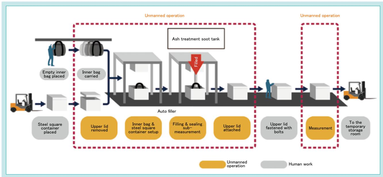
Fig. 7 Automation of Soot and Dust Filling Equipment
