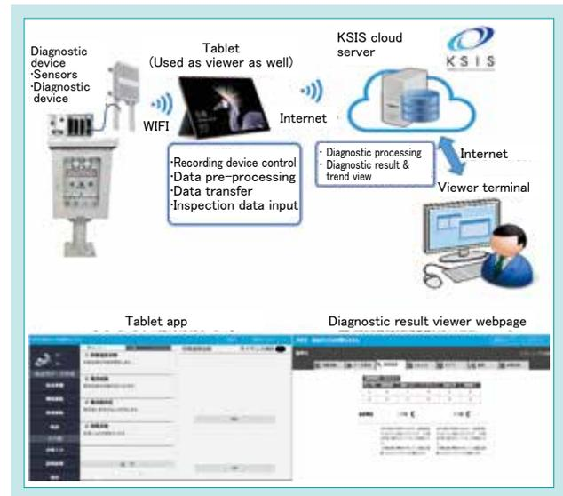
Fig. 10 Diagnostic System Configuration
