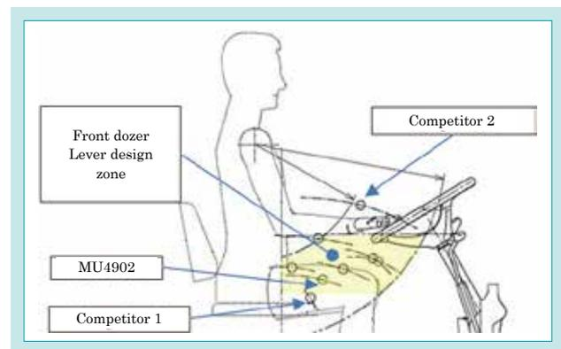
Fig. 11 Front Dozer Lever Design Zone
