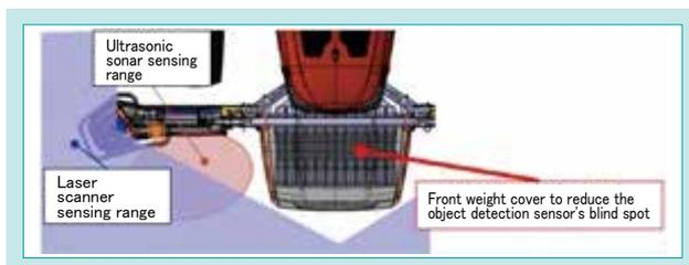
Fig. 10 Detection Area Near the Front Weight Cover
