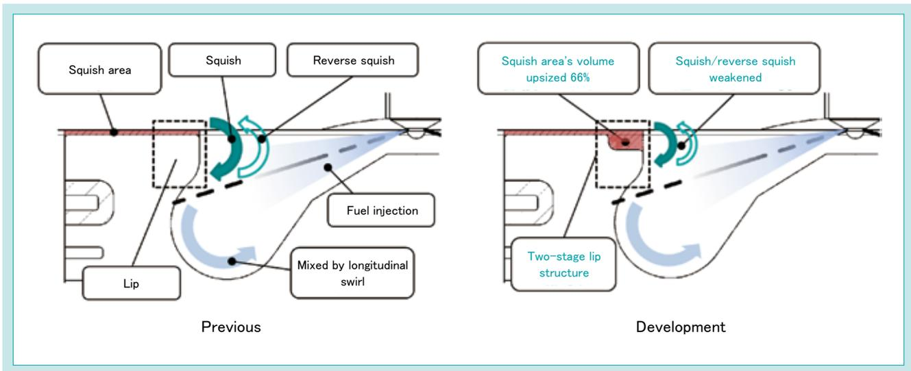
Fig. 4 Optimization of Combustion Chamber Geometry
