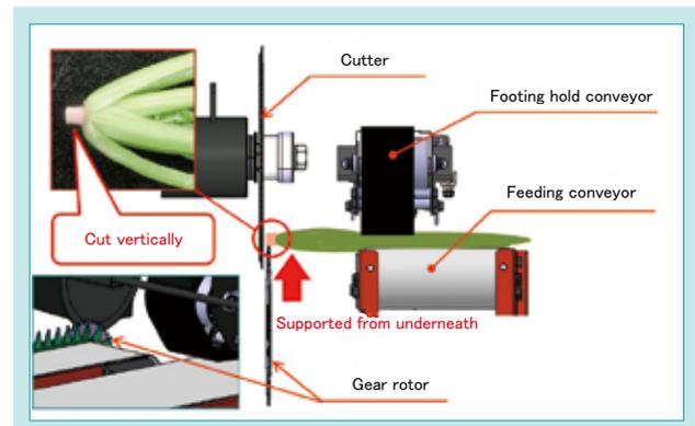
Fig. 8 Mechanism of "NC301" for Cutting Roots
