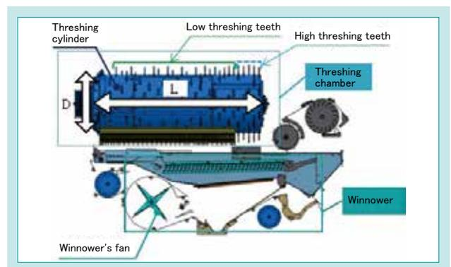
Fig. 4 Schematics of the Threshing Machine
