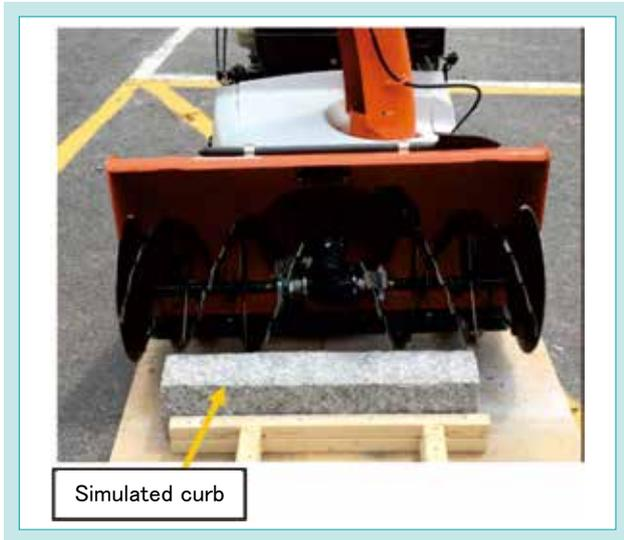
Fig. 11 Torque Limiter Operation Test
