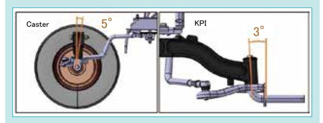
Fig. 9 T90-Series Caster and Kingpin Inclination
