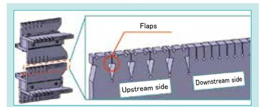
Fig. 11 Tip Shape of Blade
