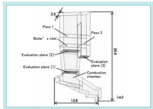
Fig. 3 Schematic of Three-dimensional Combustion Analysis Model
