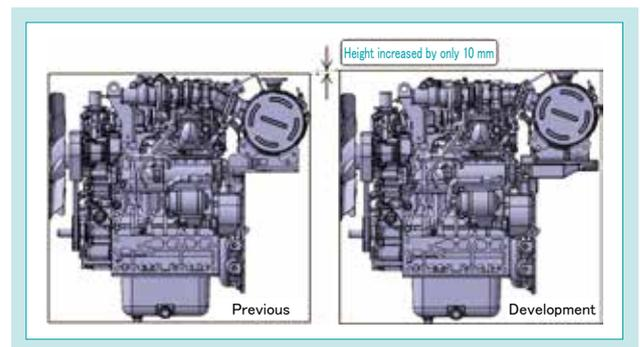
Fig. 3 Comparison of External Dimensions
