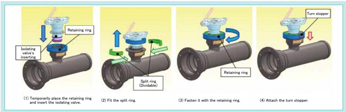
Fig. 6 Procedure for Joining
