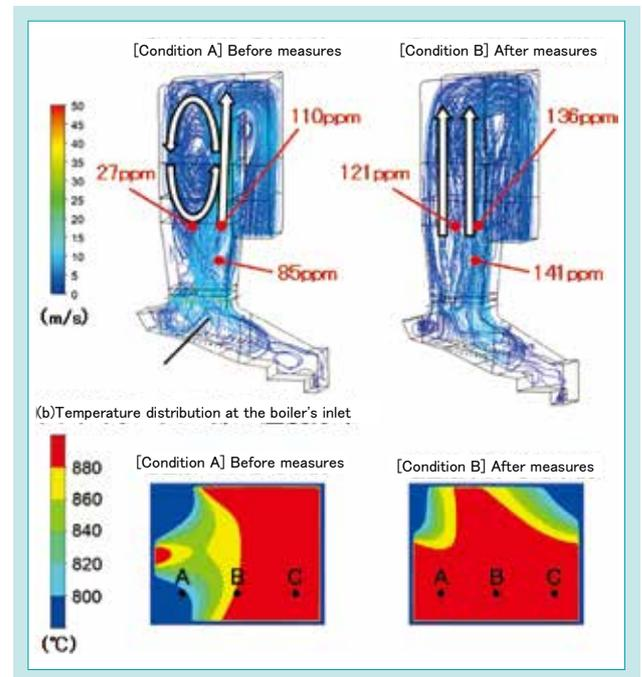
Fig. 11 Suppression Effect of Vortex Generation
