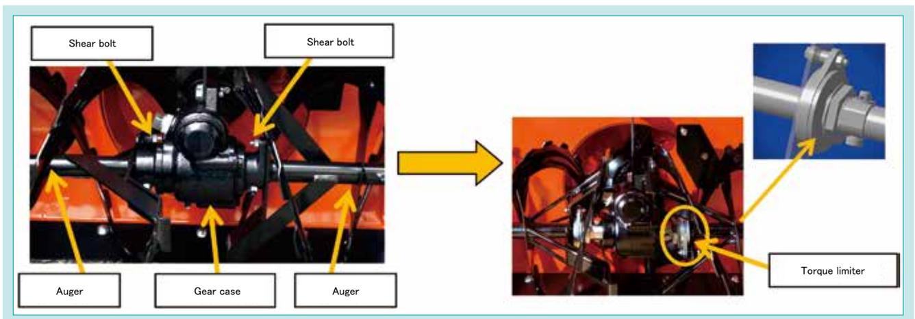
Fig. 9 Structure of Snow Removal Part
