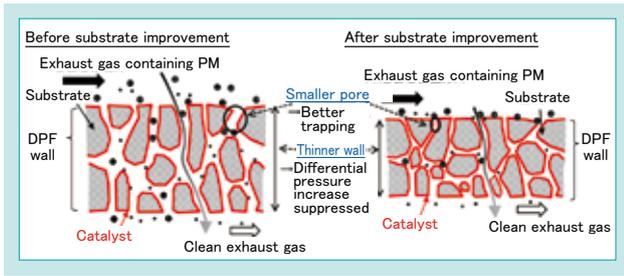
Fig. 3 Schematic Diagrams Before and After Improving the DPF Substrate
