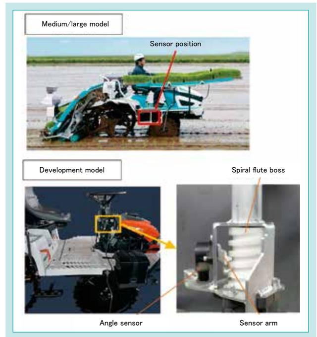
Fig. 7 Front Wheel Angle Sensor
