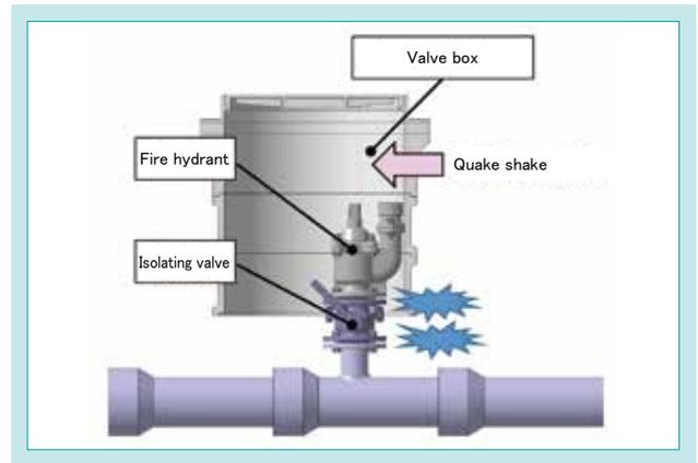
Fig. 3 Collision with Valve Box
