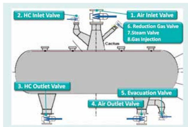
Fig. 1 SG-V Location of Reactor for PDH Plant<sup>1)</sup>
