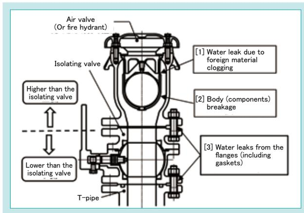
Fig. 1 Main Damage During Large Earthquake
