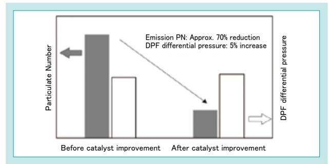
Fig. 12 PN and DPF Differential Pressures over RMC Before and After Improving the DPF Catalyst
