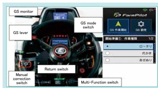
Fig. 1 SL-GS Layout, Setting Screen
