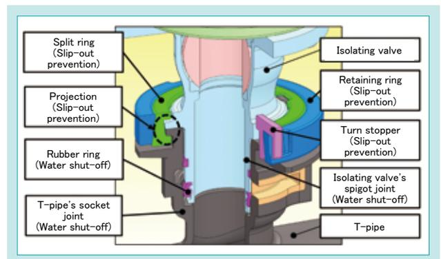
Fig. 5 Structure of Flangeless Joint
