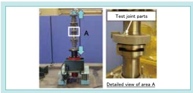
Fig. 7 Aspect of Slip-out Resistance Performance Test
