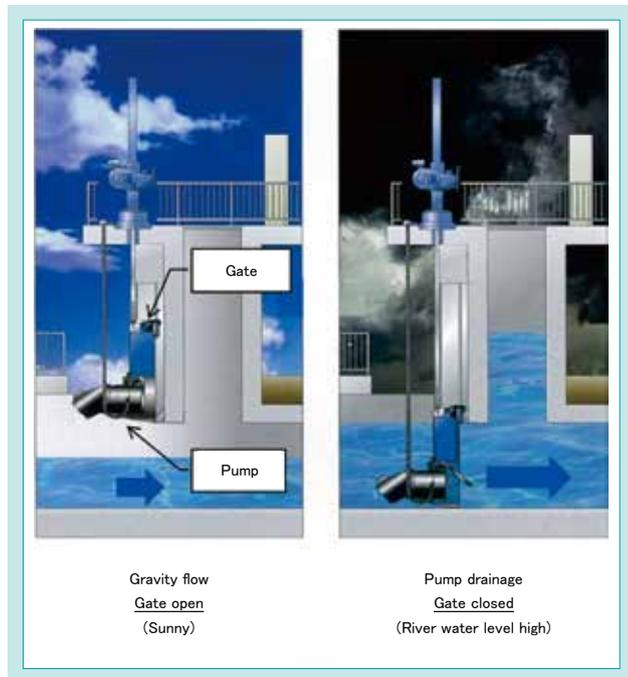
Fig. 1 Operation Method of Pump Gate
