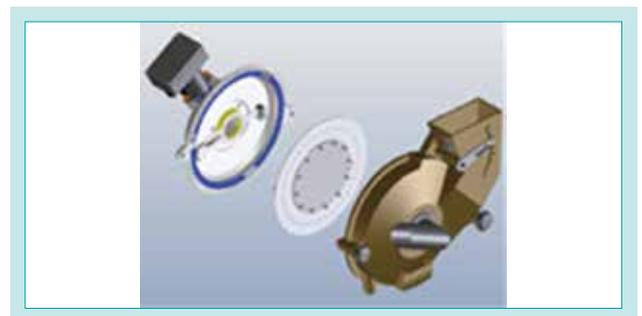
Fig. 19 Seed Heart (Drum Principle)
