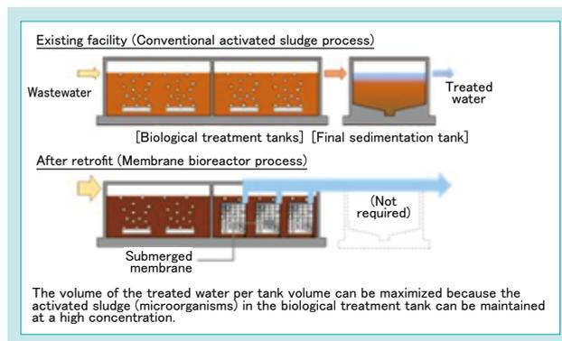
Fig. 1 Image of KUBOTA Submerged Membrane Unit Application to Retrofit of Existing Facilities
