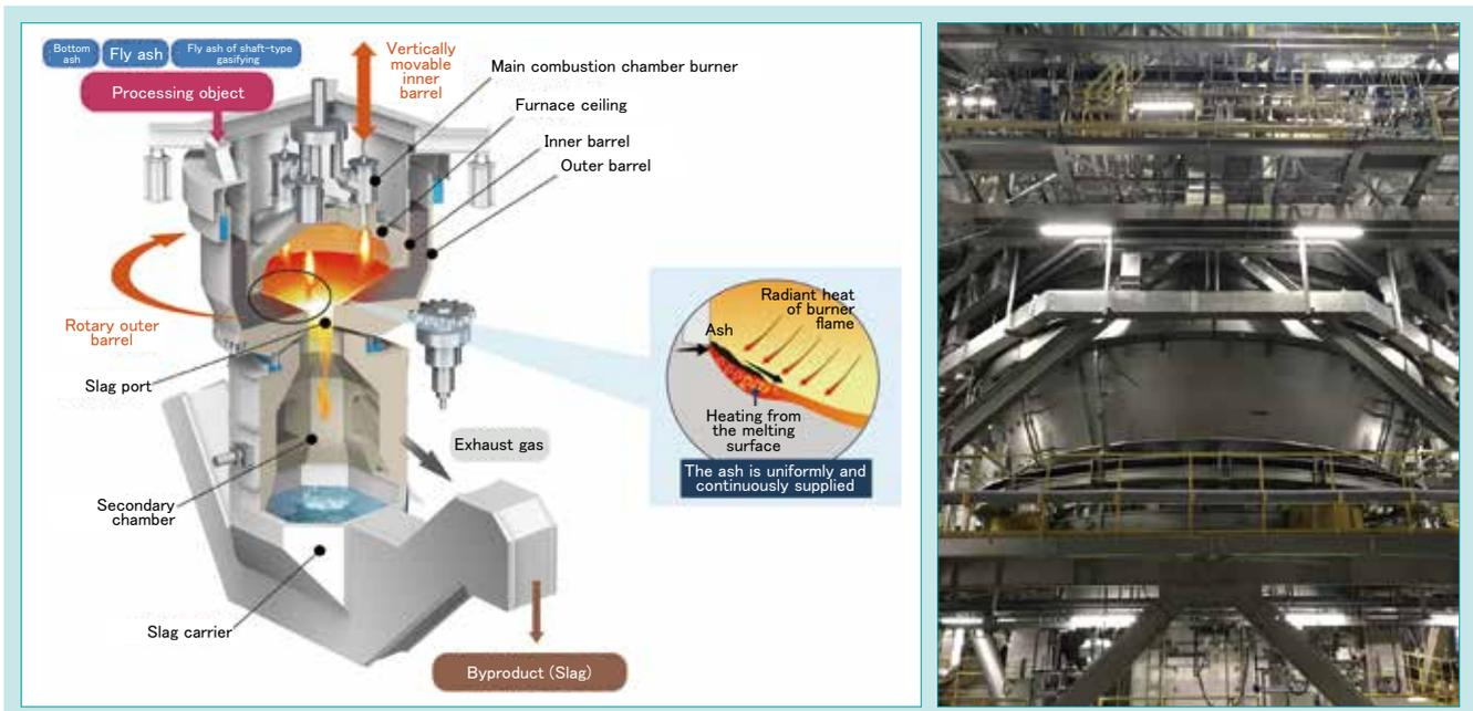
Fig. 4 KUBOTA Surface Melting Furnace
