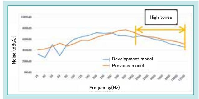
Fig. 8 Noise Frequency Comparison
