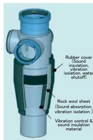
Fig. 3 Composition of Sound Insulation Material
