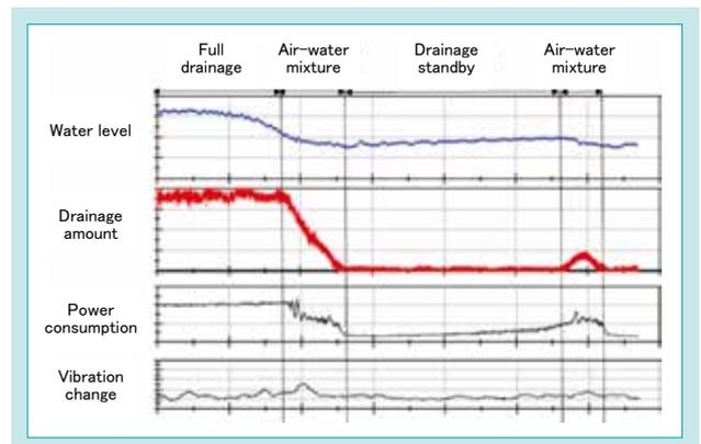
Fig. 4 Test Result of Full-speed Any-water Level Operation
