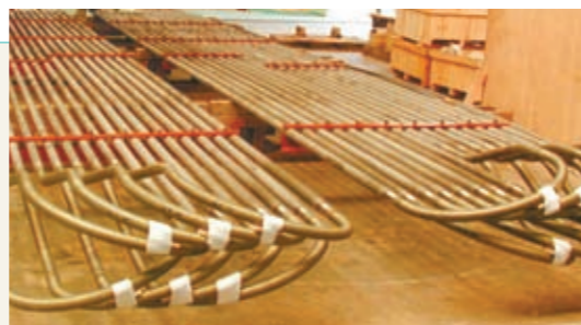
The cracking coil is an integral element of a pyrolysis furnace.
