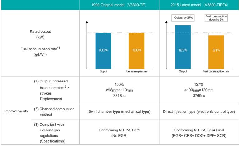
\*1 Fuel consumption rate during rated output
