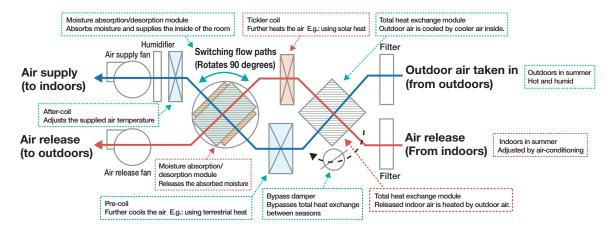
Structure of the humidity control outdoor-air processing unit and the air flows (in summer)
