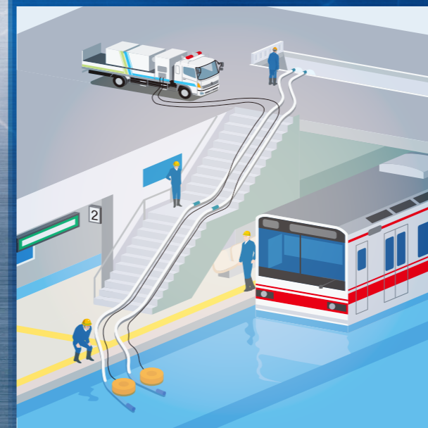
Drainage of Flooded Water at Subway
