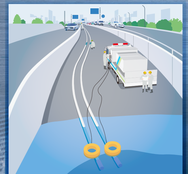
Drainage of Flooded Water at Under-Path
