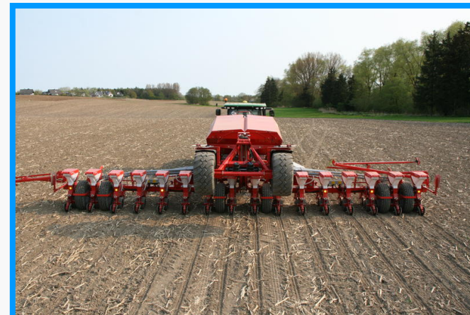
Tractor implement for corn seeding (Kverneland)
