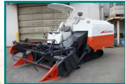
PRO688Q (for China) : Conventional-type combine harvester for rice and rapeseed
