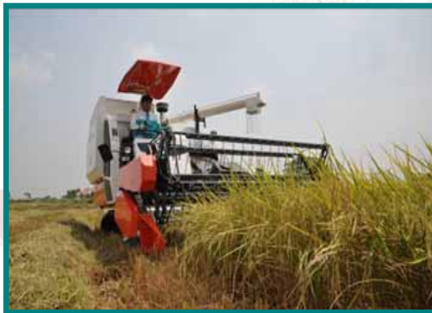
Combine harvester (Conventional type) : for harvesting rice, wheat and rapeseed.
