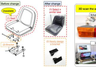
In addition to redesigning the part itself, we also conduct activities to enable substitution by selecting similar parts and designing new parts to ensure the part can be mounted compatibly.
