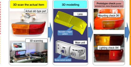
Most old-type parts do not have 3D data. We can recreate them by making a 3D scan of the actual item, then modeling it to create 3D data enabling it to be remanufactured.
