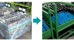
At Kubota Precision Machinery (Thailand) Co., Ltd., we revised plastic film packaging for components and changed to reusable racks, which has reduced plastic and labor.
