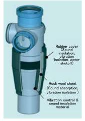
Fig. 3 Composition of Sound Insulation Material
