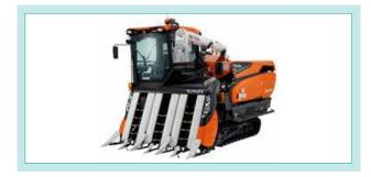
Fig. 1 Autonomous Driving Assist Combine Harvester DR6130A
