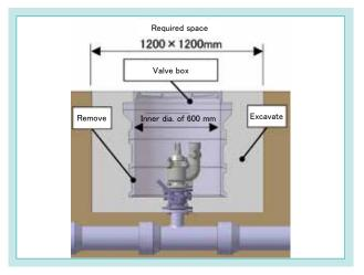
Fig. 4 Space Required for Conventional Method
