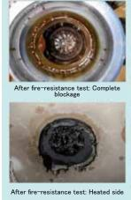
Fig. 2 Situation After Fire Resistance Test
