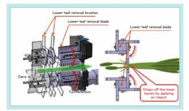
Fig. 9 Mechanism of "NC301" for Removing Cotyledons and Lower Leaves
