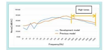
Fig. 8 Noise Frequency Comparison
