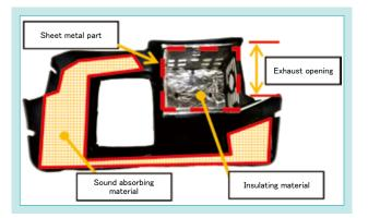
Fig. 4 Engine Top Cover Internal Structure
