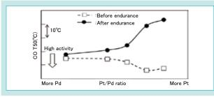
Fig. 16 CO Oxidation Activity and Pt/Pd Ratio
