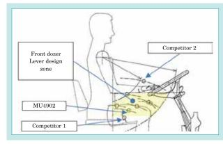
Fig. 11 Front Dozer Lever Design Zone
