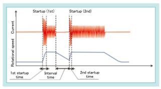
Fig. 6 Current and Rotational Speed at Pump Start-up
