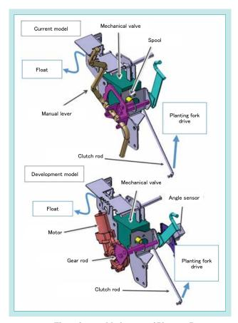
Fig. 4 Electrification Mechanism of Planting Part
