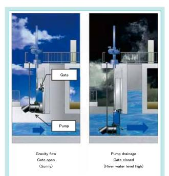
Fig. 1 Operation Method of Pump Gate
