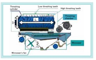
Fig. 4 Schematics of the Threshing Machine
