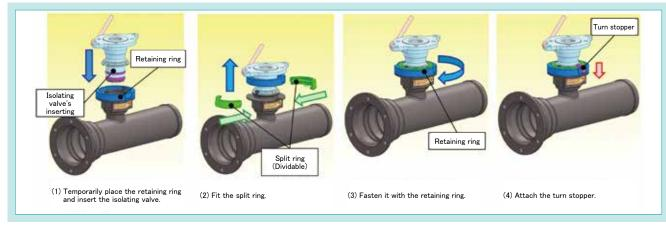
Fig. 6 Procedure for Jointing
