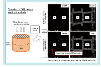
Fig. 10 EPMA and SEM Images Before and After Improving the DPF Cross Section
