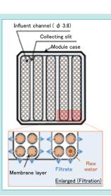
Fig. 2 Cross-section of the Flow Path
