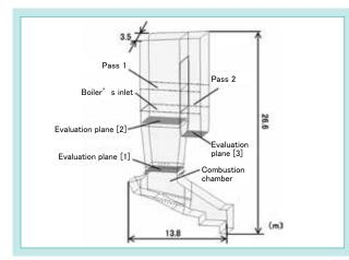
Fig. 3 Schematic of Three-dimensional Combustion Analysis Model
