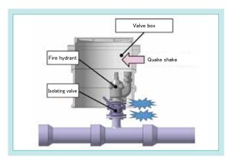
Fig. 3 Collision with Valve Box
