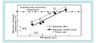
Fig. 6 Maximum Temperatures by the Thermal Shock Experiment
