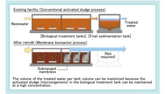
Fig. 1 Image of KUBOTA Submerged Membrane Unit Application to Retrofit of Existing Facilities
