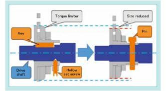
Fig. 10 Considering Miniaturization of Torque Limiter
