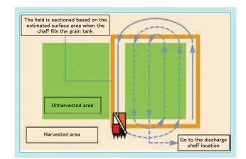
Fig. 13 Automatic Setting Area Using Yield Prediction
