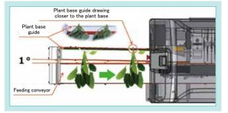
Fig. 7 Conveyor Arrangement of the Feeding Unit of "NC301"
