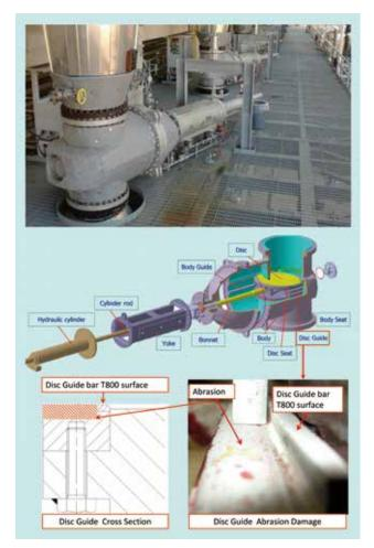
Fig. 3 Overview of Special Gate Valve and Typical Damage
