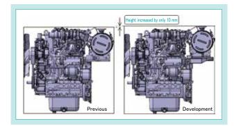
Fig. 3 Comparison of External Dimensions
