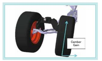
Fig. 10 T90 Camber Gain in a Turn
