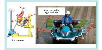
Fig. 5 Line Marker for Medium and Large Class
