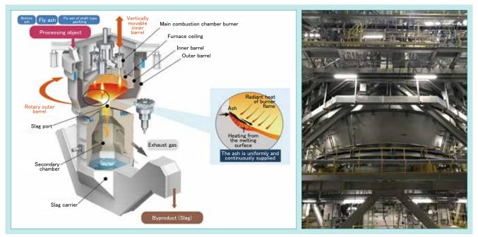
Fig. 4 KUBOTA Surface Melting Furnace
