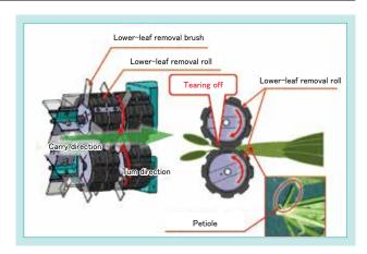
Fig. 6 Mechanism of "NC300" for Removing Cotyledons and Lower Leaves
