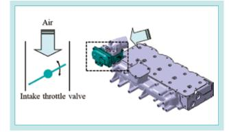
Fig. 7 Intake Throttle Valve
