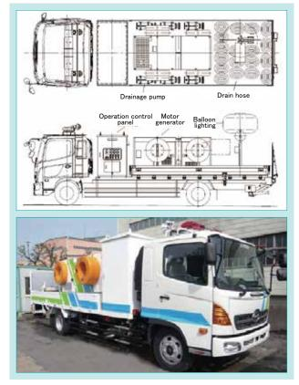
Fig. 4 Current Drainage Pump Vehicle
