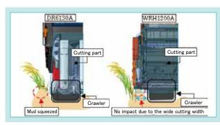
Fig. 10 Relative Position Between Reaper and Crawler
