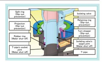
Fig. 5 Structure of Flangeless Joint
