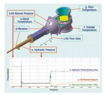
Fig. 4 Extracted Target Data for Measurement
