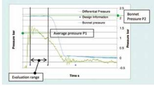
Fig. 6 Evaluation Factor for Valve Sealing Function
