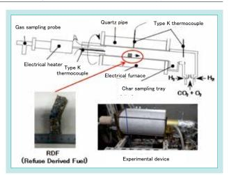
Fig. 2 RDF Combustion Test Device
