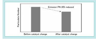
Fig. 17 PN Results over RMC Using Less Aged DPF
