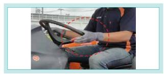
Fig. 8 Position of Shuttle Lever
