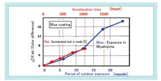
Fig. 4 Comparison of Change in blue color between Miyako (blue) and Xenon (red)
