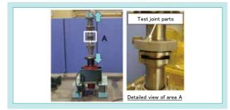
Fig. 7 Aspect of Slip-out Resistance Performance Test
