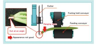
Fig. 5 Mechanism of "NC300" for Cutting Roots
