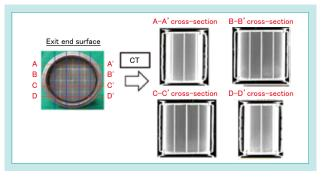
Fig. 7 CT Images for the DPF After Diesel Engine Endurance Test
