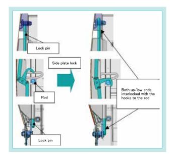
Fig. 8 Locking Mechanism
