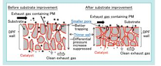
Fig. 3 Schematic Diagrams Before and After Improving the DPF Substrate
