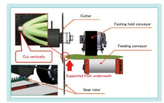
Fig. 8 Mechanism of "NC301" for Cutting Roots
