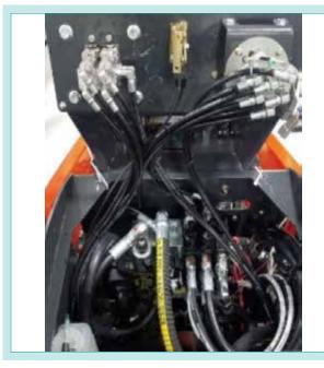
Fig. 3 Hydraulic Hose Routings
