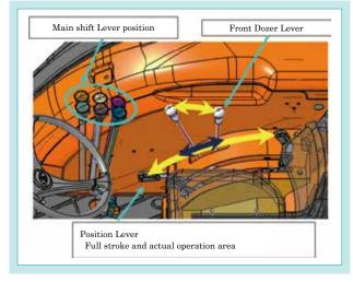
Fig. 10 Positioning of Operating Levers
