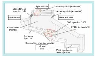
Fig. 4 Positions of Gas Injection Ports
