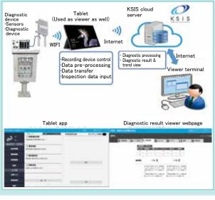
Fig. 10 Diagnostic System Configuration
