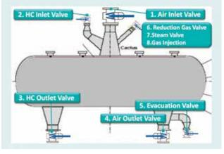
Fig. 1 SG-V Location of Reactor for PDH Plant<sup>1)</sup>
