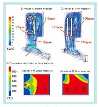
Fig. 11 Suppression Effect of Vortex Generation
