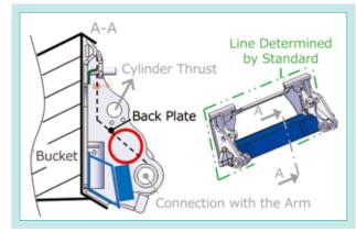
Fig. 10 Structure of Hitch
