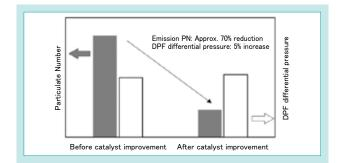
Fig. 12 PN and DPF Differential Pressures over RMC Before and After Improving the DPF Catalyst
