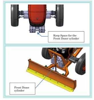
Fig. 4 Positioning of Front Weight and Front Dozer
