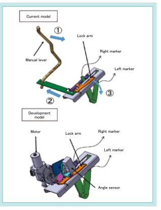
Fig. 6 Electrification Mechanism of Line Marker
