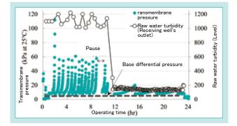
Fig. 7 Transmembrane Pressure During High Turbidity Test
