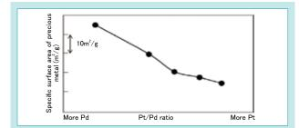
Fig. 15 Surface Area for Noble Metal and Pt/Pd Ratio
