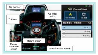
Fig. 1 SL-GS Layout, Setting Screen
