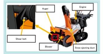
Fig. 1 Two-stage Snow Blower SLA-1070A
