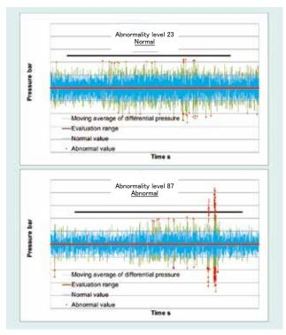
Fig. 5 Evaluation Factor for Valve Operating Function
