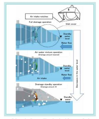
Fig. 3 Relationship Between Water Level and Operating Condition
