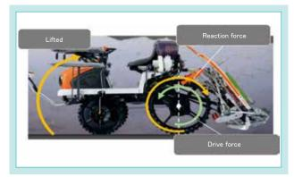
Fig. 9 Lifting of the Body due to Load
