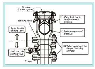
Fig. 1 Main Damage During Large Earthquake
