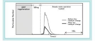
Fig. 11 PN after DPF Regeneration Before and After Improving the DPF Catalyst
