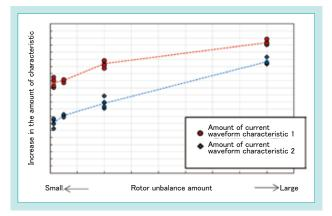
Fig. 8 Effect of Pump Rotor Unbalance
