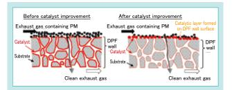
Fig. 9 Schematic Diagrams Before and After Improving the DPF Catalyst
