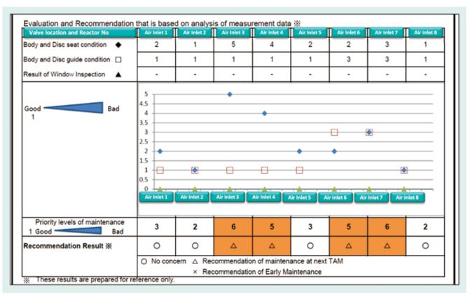
Fig. 8 Priority Level Sample for Maintenance
