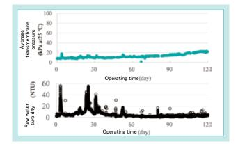
Fig. 6 Mean Transmembrane Pressure During Long Time Operation
