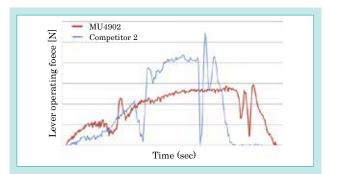
Fig. 9 Operating Force of Shuttle Lever
