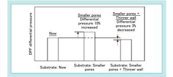
Fig. 4 DPF Differential Pressures Before and After Improving the DPF Substrate
