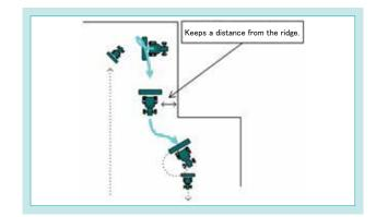
Fig. 4 Turning Route Along the Ridge
