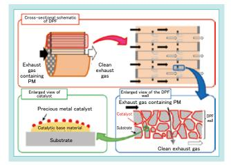
Fig. 2 Schematic Diagrams of a DPF
