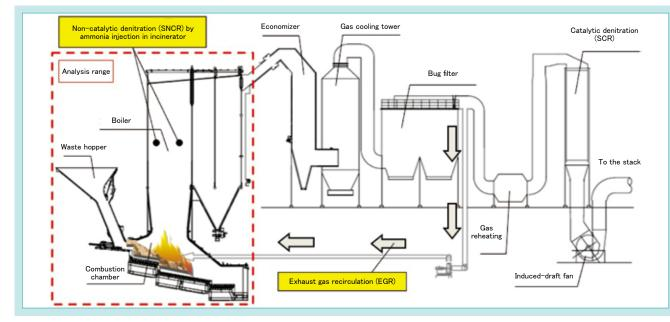
Fig. 1 Outlined Scheme of the Municipal Waste Incinerator
