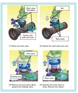
Fig. 10 Replacement Method Procedure
