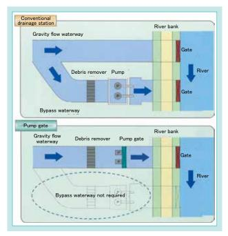
Fig. 2 Shape of Conventional Drainage Pump Station and Pump Gate
