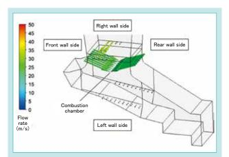
Fig. 8 Velocity Vectors Around Secondary Air-injection Ports
