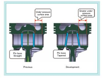
Fig. 6 Tapered Pin Boss
