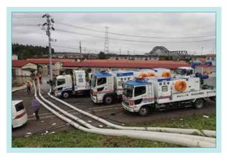
Fig. 1 Drainage Pump Vehicles Operating Photo
