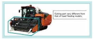
Fig. 3 Autonomous Driving Assist Combine Harvester WRH1200A
