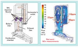
Fig. 6 Scheme of SNCR Test in Actual Incinerator
