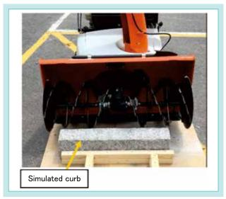
Fig. 11 Torque Limiter Operation Test
