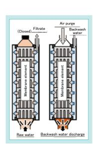
Fig. 3 Internal Flow of the Module
