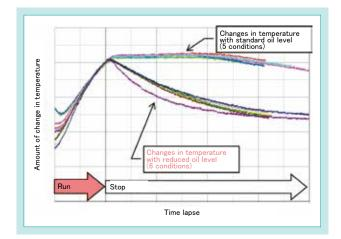
Fig. 9 Lubricating Oil Temperature of Mechanical Seal
