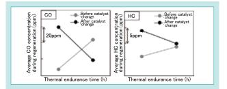
Fig. 19 CO and HC Emissions During DPF Regeneration
