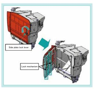
Fig. 7 Easy Maintenance of Grain Tank
