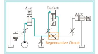
Fig. 16 Hydraulic Circuit 5(AMV)
