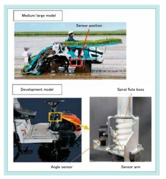
Fig. 7 Front Wheel Angle Sensor
