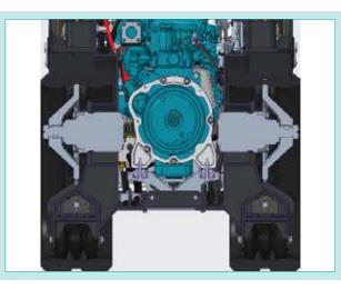
Fig. 2 Drive Sprockets and Motors
