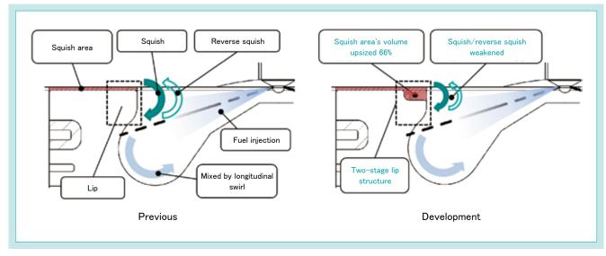
Fig. 4 Optimization of Combustion Chamber Geometry
