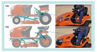
Fig. 12 T80 vs T90 Mower Lift Operation
