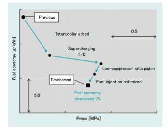
Fig. 5 Suppression of Pmax and Improvement of Fuel Efficiency
