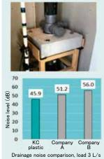
Fig. 4 Noise Measurement Result
