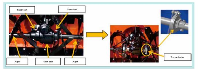
Fig. 9 Structure of Snow Removal Part
