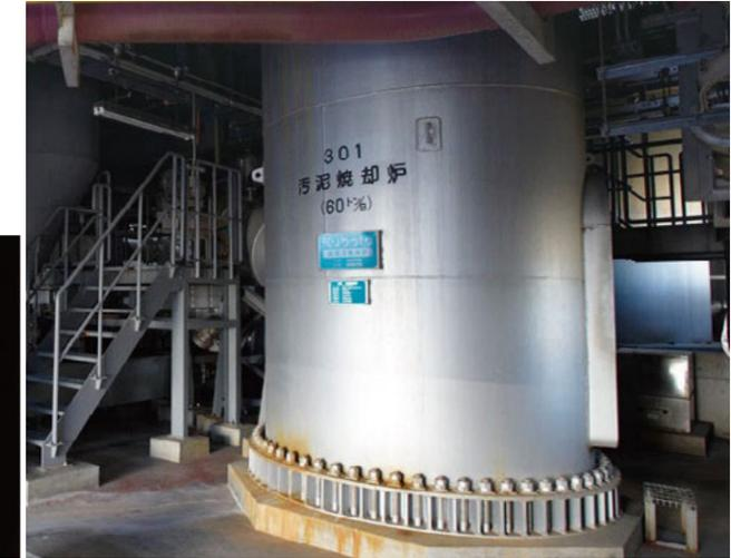
Circulating fluidized bed incinerator (base)
