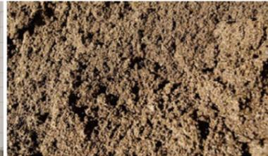
Hamamatsu City Seibu Waste Incineration Plant – a portion of the dewatered sludge is co-combusted with garbage in the waste incineration plant's combustion/melting furnace to create sand-like slag (bottom photo) that can be used as a material for asphalt.
