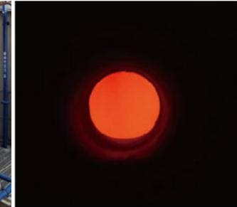
Interior of the incinerator as seen from the viewing window. By switching from ordinary incineration (800°C) to high-temperature incineration (850°C), the circulating fluidized bed incinerator can reduce N<sub>2</sub>O emissions by approximately 60%.
